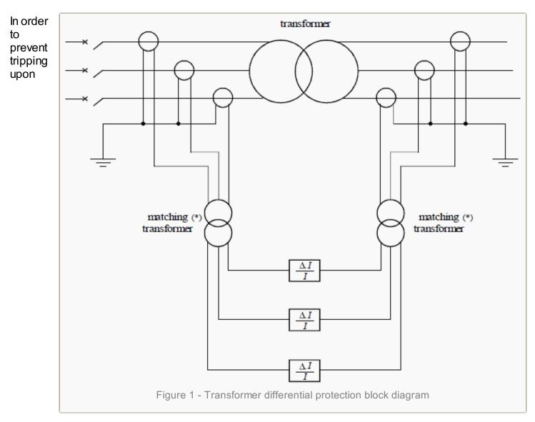
occurrence of high fault currents of external origin, biased differential protection devices are used.
